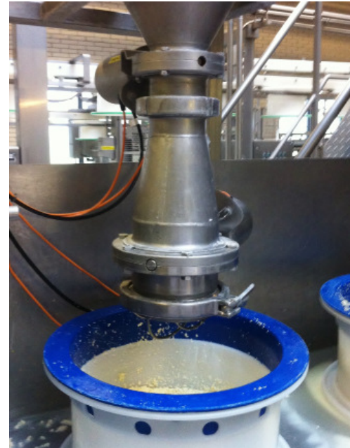
Cheese grains are returned to moulds on the production line subsequent to collection and filtering.
