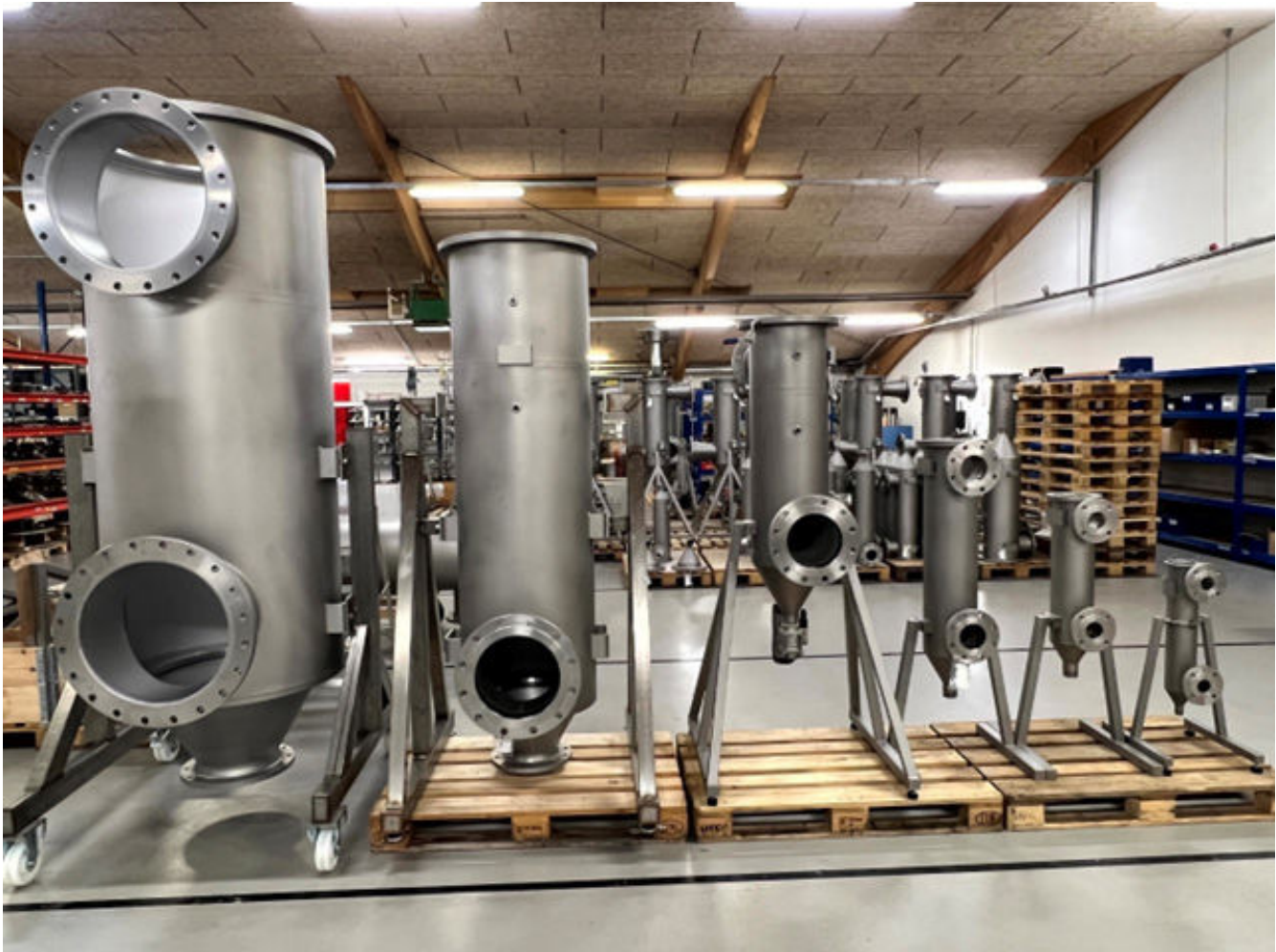
Image 2: The self-cleaning filter solutions have significantly grown in recent years. Far left is the gigantic Auto-line LVLR filter, setting new standards when it comes to flow. The filter has a capacity of 2000 cubic meters of water per hour.
