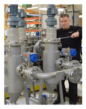
The finishing touches are made to the two-stage filter for coffee production in India. A customised solution service is provided to locations across the world from the company's Hedensted base.
