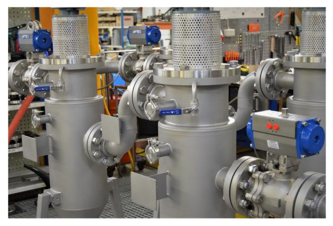
One filter ensures fine filtration of the coffee, the other coarse filtration. The solution runs on two lines simultaneously, meaning use of four filters in total.
