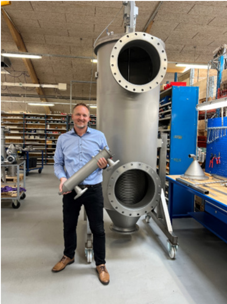
A large and a small one. Martin Holgaard, Sales Director at HiFlux Filtration A/S, next to the company's largest filter ever. The new Auto-line LVLIR filter can process 2000 cubic meters of water per hour, and the filter housing is over four meters in height.
