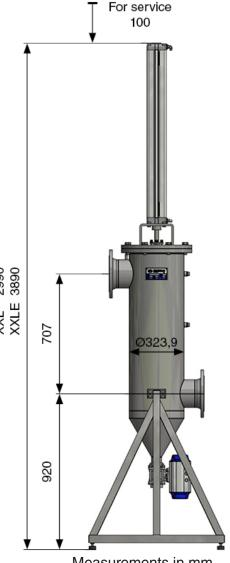
Measurements in mm.
