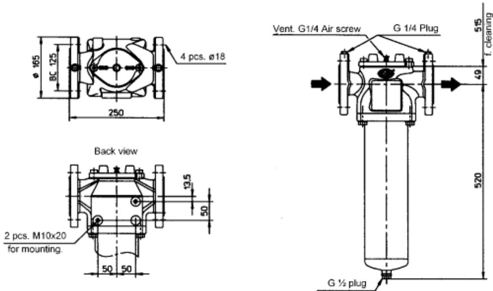
HiFlux Micro-line 1050 is manufactured in EN-GJS-500-7 cast iron and stainless acid-proof EN 1.4404 steel and accomodates current standards and norms for pressure vessels.
